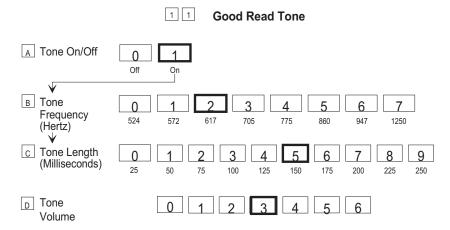
Note: When entering Tone Frequency, Tone Length, or Tone Volume, the adjustment can be incremented upward by scanning the **Hex A** tag. Each time you scan the **Hex A** tag, the selection increases one unit. Scan the **End** tag or a valid Hex tag to end this mode of input.
