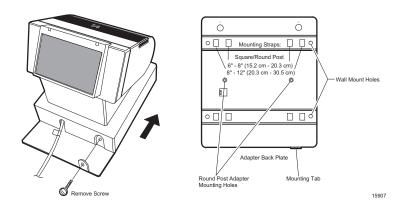
**Note:** If you are mounting to a hollow wall, such as drywall, use a 3/16 inch diameter (or larger) toggle bolt.
